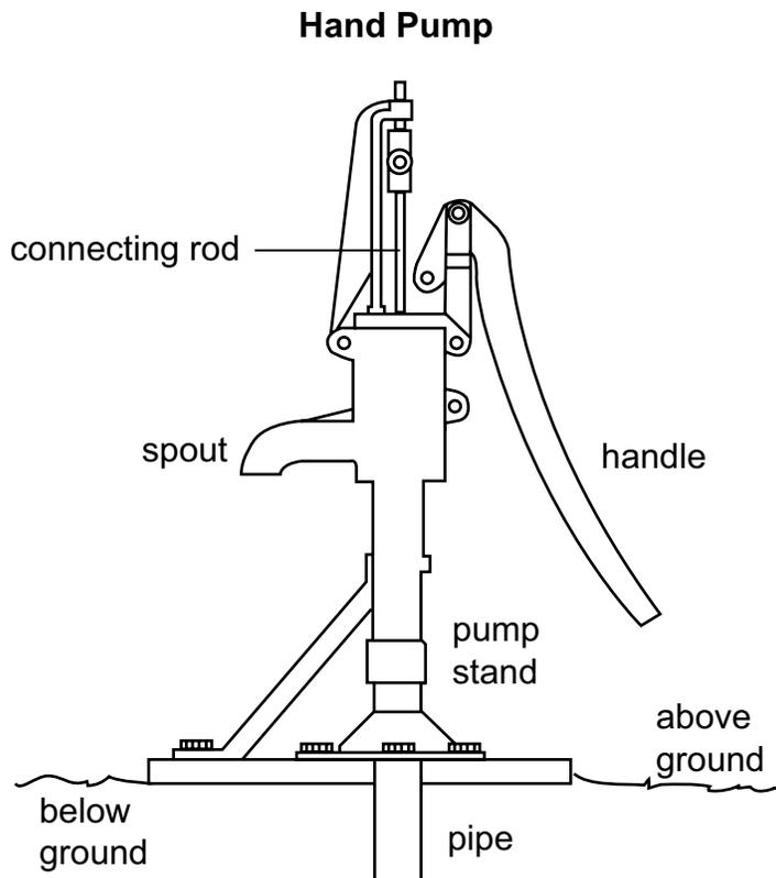
The diagram shows a type of hand pump used to bring water up from below the ground. Which flaw in the pump keeps it from functioning properly?
