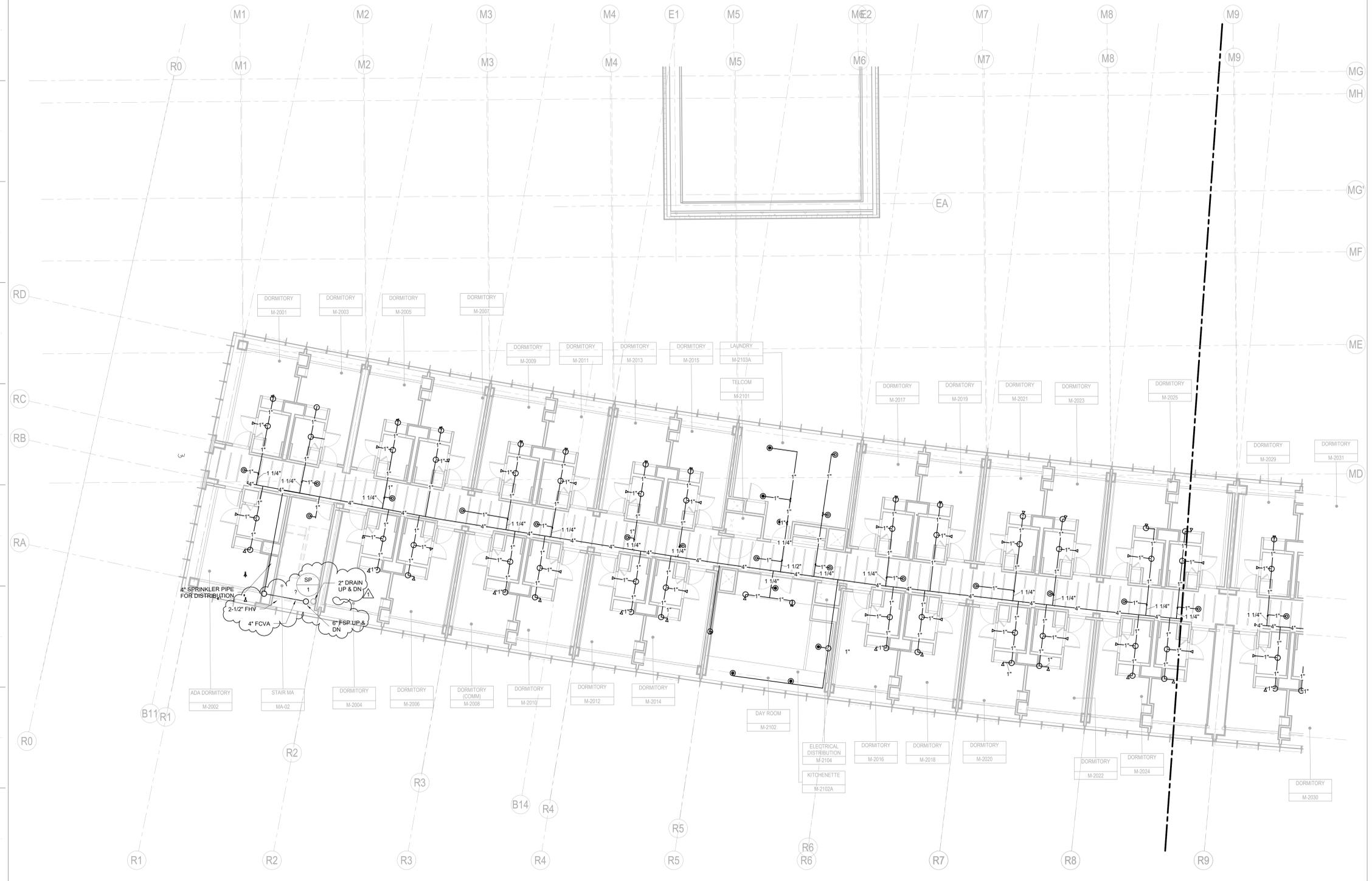
**1 MARQUEE - FLOOR PART PLAN A - LEVEL 3 - FIRE PROTECTION**
